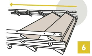
Tip: repeat the measurements regularly and adjust the length of the blades if the structure is not perfectly parallel.
