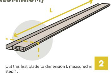
For aluminum: cut with a fine multi-toothed blade. **Remember to wear goggles and gloves.**
